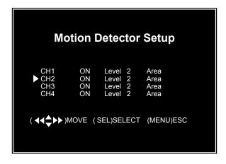
This sub-menu allows you to set the motion detection options for each camera.
